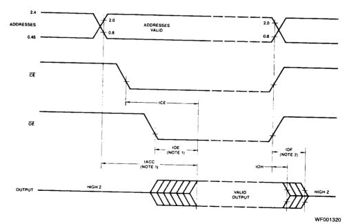
Notes: 1.  $\overline{OE}$  may be delayed up to  $t_{ACC}$  -  $t_{OE}$  after the falling edge of  $\overline{OE}$  without impact on  $t_{ACC}$ . 2.  $t_{DF}$  is specified from  $\overline{OE}$  or  $\overline{CE}$ , whichever occurs first.
