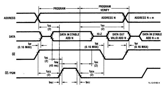
Note: All times shown in parentheses are minimum times and are in  $\mu s$  unless otherwise specified.
