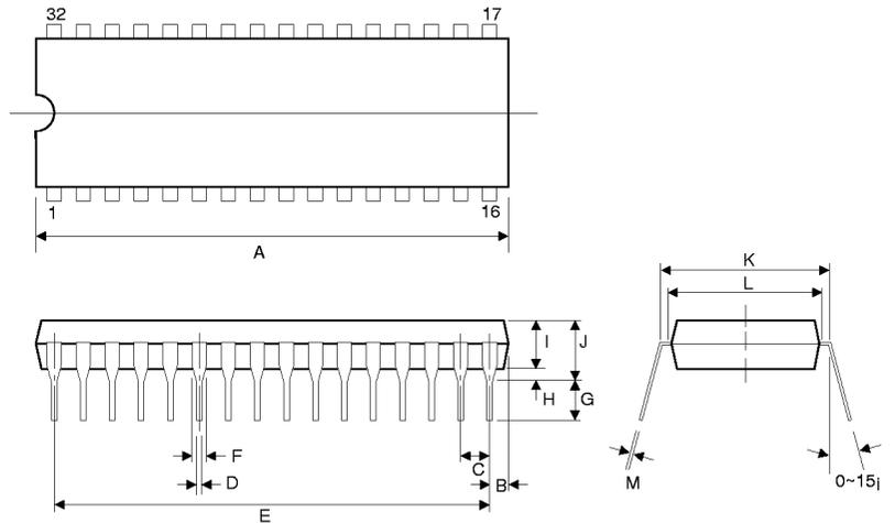
**NOTE:** Each lead centerline is located within .25 mm[.01 inch] of its true position [TP] at maximum material condition.
