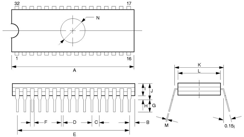
**NOTE:** Each lead centerline is located within .25 mm[.01 inch] of its true position [TP] at maximum material condition.
